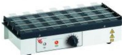
The Slide Drying Bench aids in the preparation of microscope slides at the specimen mounting stage. It complements both the Paraffin Wax Dispenser and the Paraffin Wax Mounting Bath to provide a complete set of paraffin wax sampling equipment for the modern laboratory.
